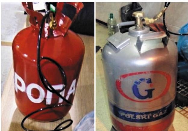
Testing of the cylinders with a refrigerant identifier showed that the cylinder labelled "propane" actually contained HFC-134a, and the cylinder without labeling contained HFC-404A. Pursuant to the EU and national legislation, both cylinders were sent back to the country of dispatch.
