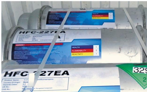
Labelling of cylinders containing HFC-227ea, a controlled chemical used as fire suppressant, foam blowing agent and increasingly in new refrigerant blends to suppress the flammability of the other components, e.g. R-461 or R-470. This labelling provides information on the safety of transport like the UN number and dangerous goods label. It also includes the chemical name and safety warning as required by the legislation on chemicals.
