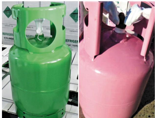
As per the customs declaration, the green cylinders contained HFC-134a and the pink cylinders HFC-410A. Lack of labelling did not allow for the identification of the substances once the cylinders were taken out of the cardboard boxes. Before release for free circulation, the cylinders had to be labelled in compliance with the EU F-gas legislation and the legislation on chemicals.
