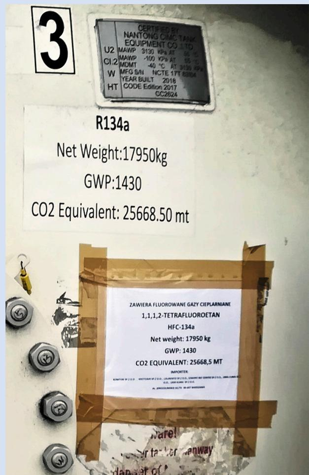
Taped paper label on an ISO tank with an additional statement in Polish reading "Contains fluorinated greenhouse gases", which is a requirement of the EU F-gas legislation
