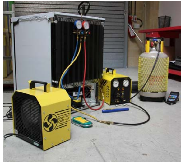
Figure 5, Example of equipment used for servicing HC systems
