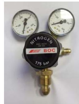
Figure 9, appropriate regulator for pressure testing R744 systems
