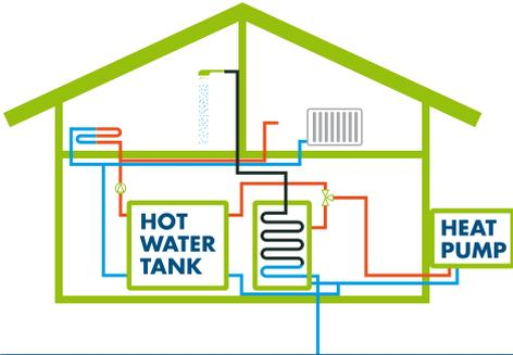
**Heat pumps** are much **more efficient** than other forms of heating and are widely used: **they extract energy from air or water and transfer it to heat homes and office buildings.** Compared to direct heating with fossil fuels they are much more energy efficient.
